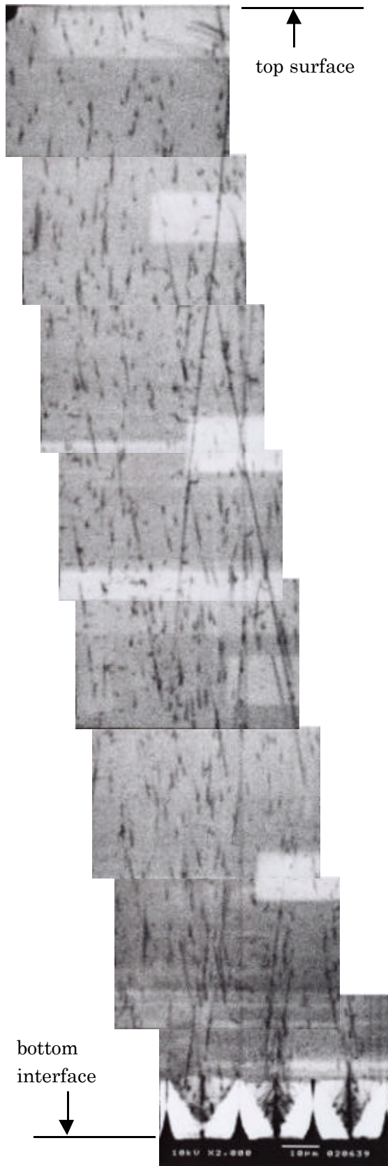
Fig. 5 Cross-sectional CL images from the top surface region to the bottom interface, including the seed region of GaN/sapphire interface of a freestanding GaN wafer
